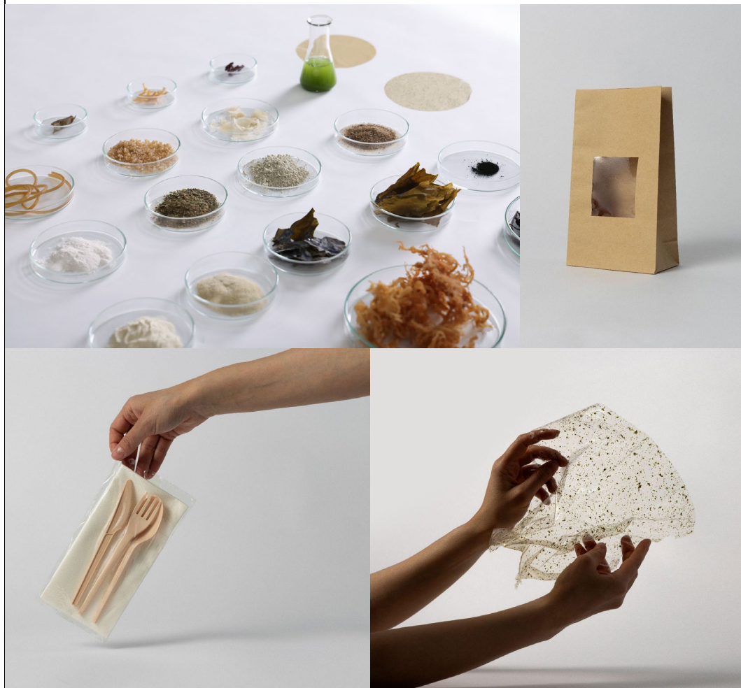
Figure 10: A selection of raw materials and processed seaweed-based materials (top-left), viewing window made out of seaweed-based materials for cardboard packaging (top-right), transparent packaging film for cutlery packaging (bottom-left), noriware’s seaweed-based packaging film (bottom-right).
